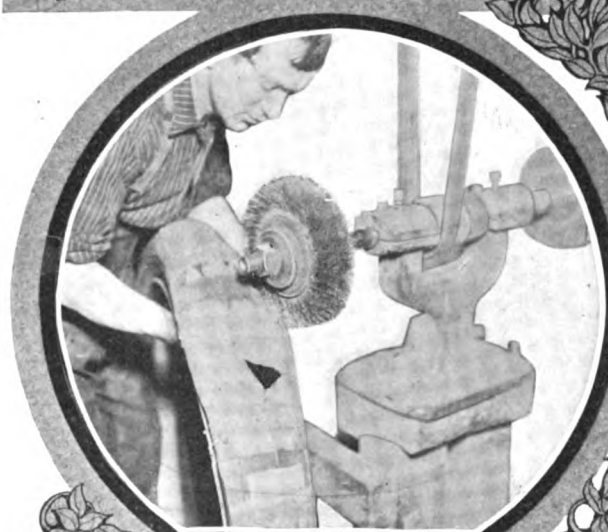
E—Buffing bad places before rebuilding
